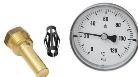
Bimetallic thermometer TT 60 is intended for temperature measurement in hot water or steam distribution systems. The minimum temperature is 0 °C. The thermometer must be installed in thermometer well.
